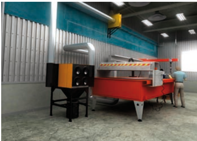
MultiDustBank, TEV fan and DCV/TG-controller connected to a cutting table
